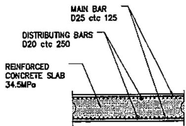
CONCRETE SLAB SECTION
